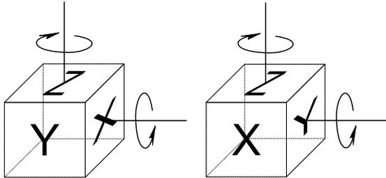
Figure 9: Excitation of three directions with a two axis system
