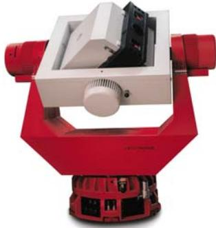
*Figure 4: Three Axis Simulator with Thermal Vacuum Chamber*
