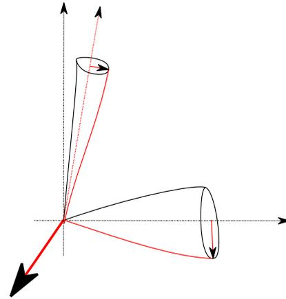
Figure 13: Wobble-, Orthogonality- and Position error constitute the pointing accuracy
