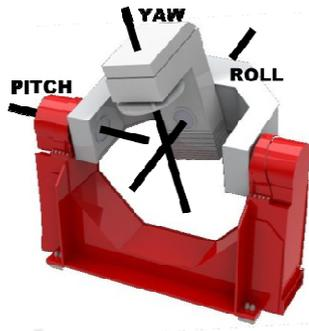
Figure 6: Axis Sequence for Optronics Testing
