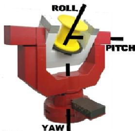
Figure 7: Classical axis orientation for IMU testing
