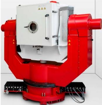
Figure 2: Three Axis Simulator with Temperature Chamber
