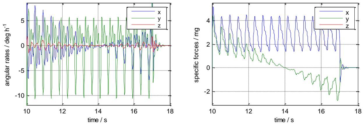
Figure 6: Resulting UUT motion caused by a walking human.
