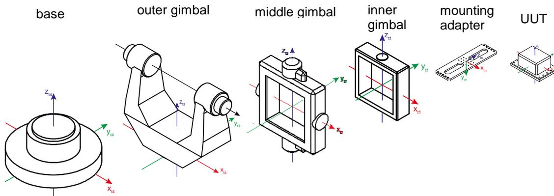
Figure 8: Three axis motion simulator multi-body model.
