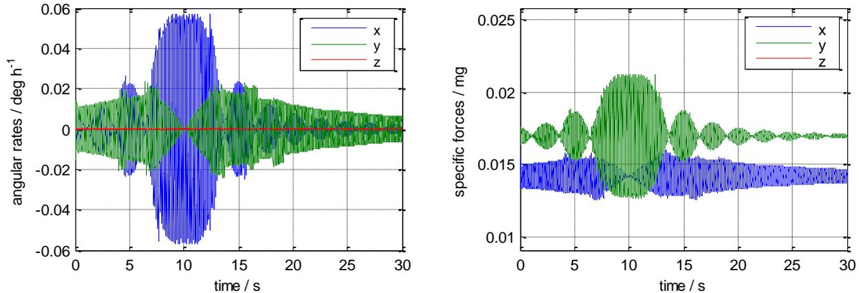
Figure 5: Resulting UUT motion caused by a passing truck.
