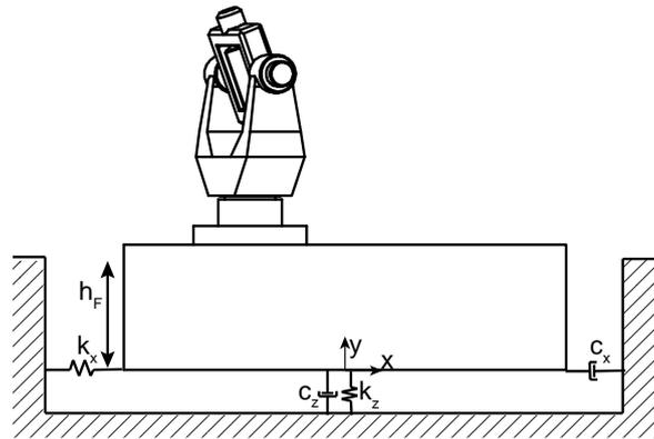
Figure 3: Model of foundation and soil interaction.
