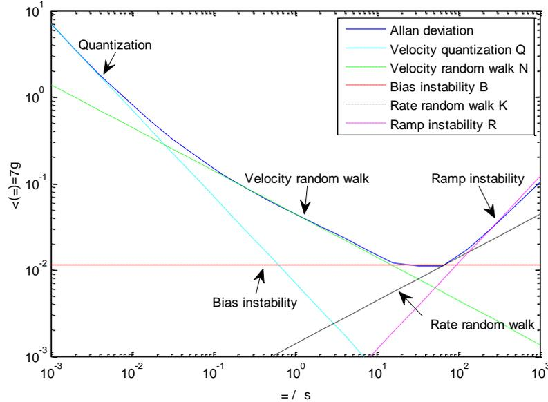
Figure 10: Synthesis of an accelerometer noise model.
