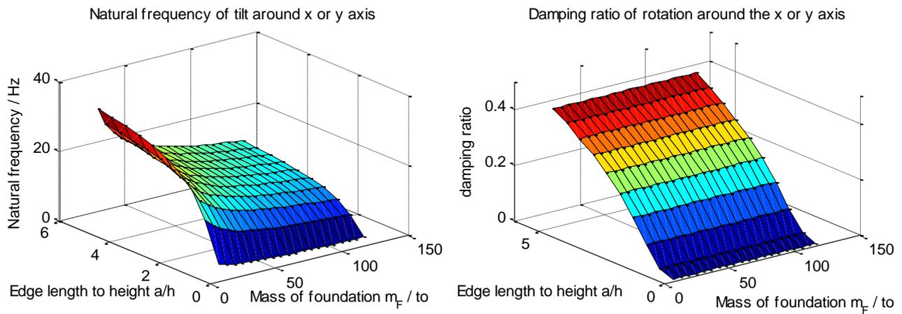
Figure 4: Influence of foundation dimensions on oscillation characteristics.
