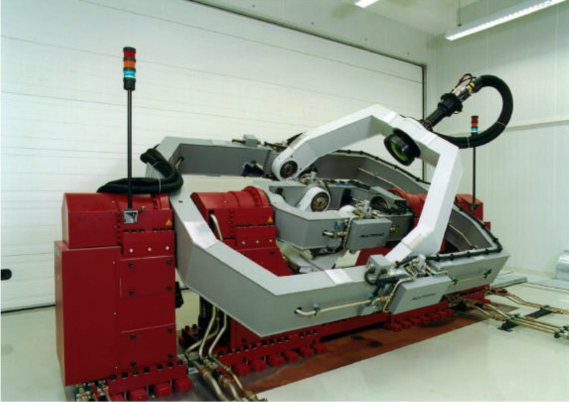
Figure 1-1 Photograph of Acutronic Model HD7756 Flight Table Showing Simulation Elements at the Daimler Chrysler Aerospace LFK HWIL Laboratory
