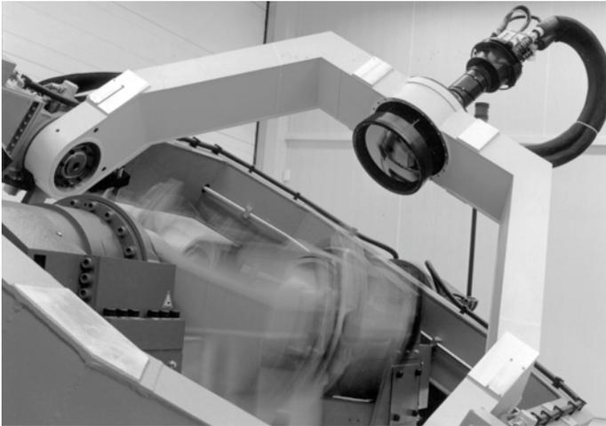
**Figure 1 : Flight Motion Simulator in operation**
