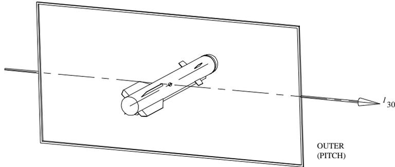
Figure 4-8: Inertia Definition for Outer (Pitch) Axis
