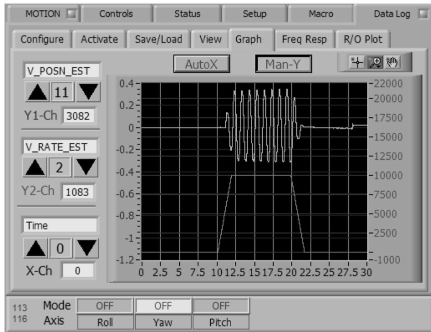
Figure 4-9: Position Disturbance On Pitch Axes Caused By Gyroscopic Torques
