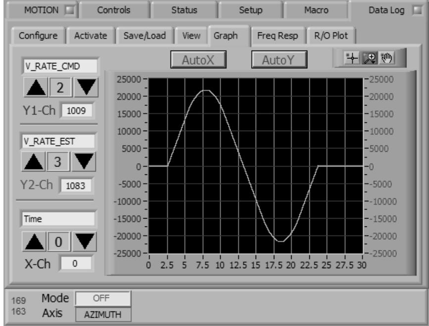
Figure 5-2: Peak Speed Measurement of AC130HS High Speed Roll
