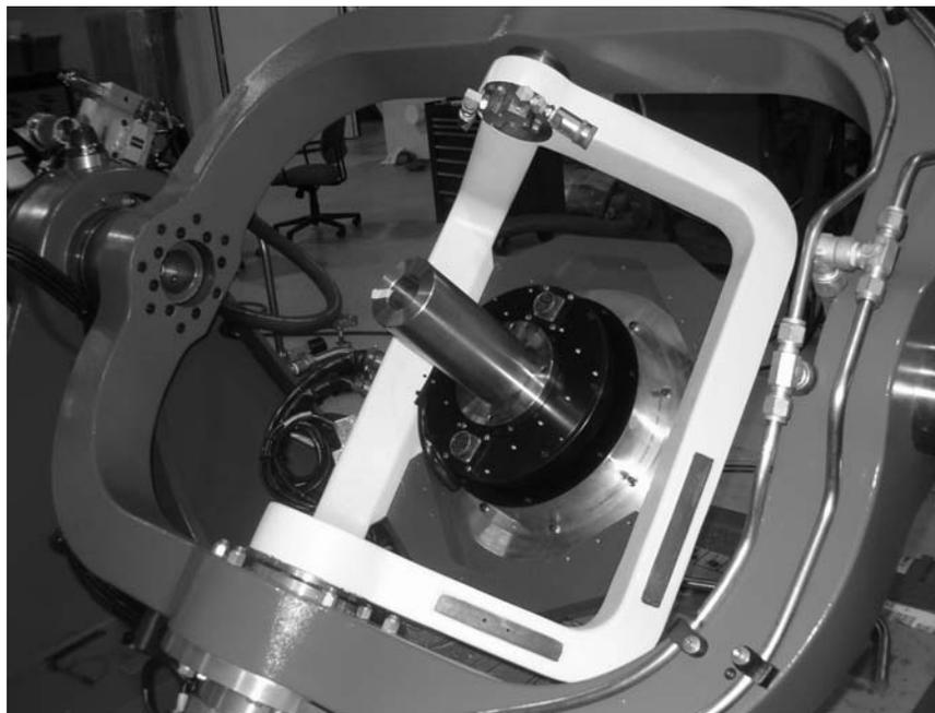
Figure 4-1: AC130HS High Speed Roll Drive Mounted to a Carco S450 Flight Motion Simulator
