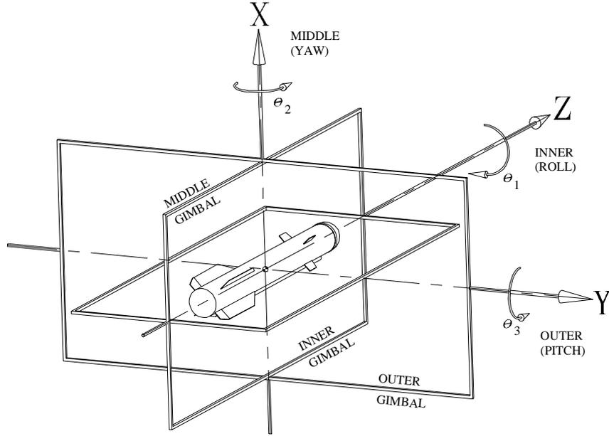
Figure 4-5: Coordinate Convention for Flight Motion Simulator
