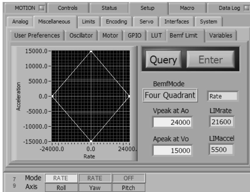
Figure 4-4: Acutrol3000 Torque vs. Speed Limitations for Trajectory Generation
