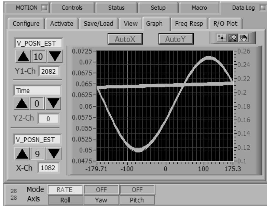
Figure 4-10: Yaw Axis Position Disturbance When Roll Is Operated At 10,000 Deg/Sec And An Imbalance Of 1.6 Oz At 4.0 In Is Attached To The Tabletop
