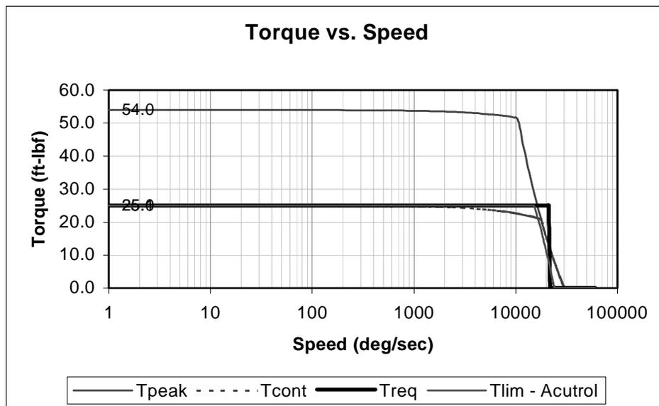
Figure 4-2: Torque vs. Speed Curve for AC130HS High Speed Roll Drive Option
