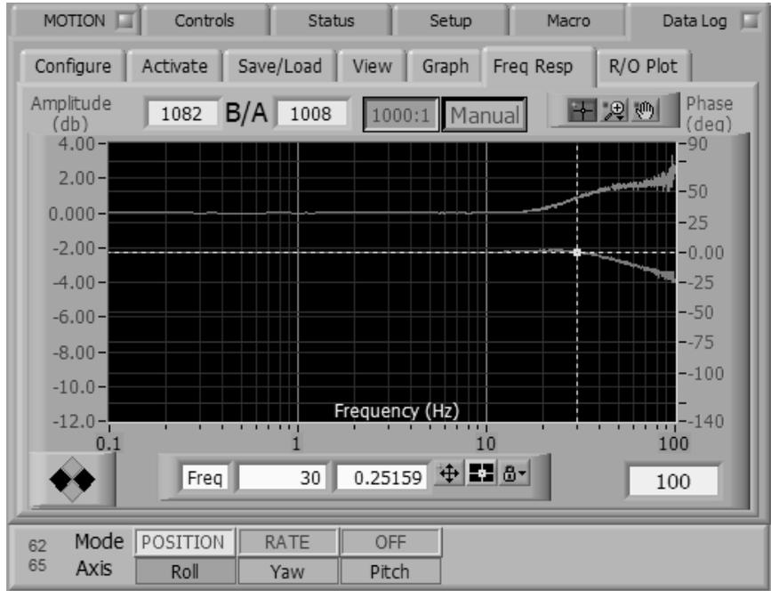
Figure 5-1: Frequency Response of AC130 HS High Speed Roll Drive showing only 2 dB of Gain and 25 deg of Phase Lag at 100 Hz
