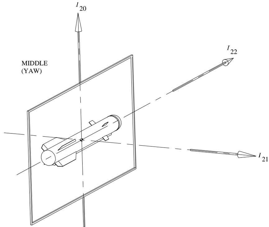
Figure 4-7: Inertia Definition for Middle (Yaw) Axis
