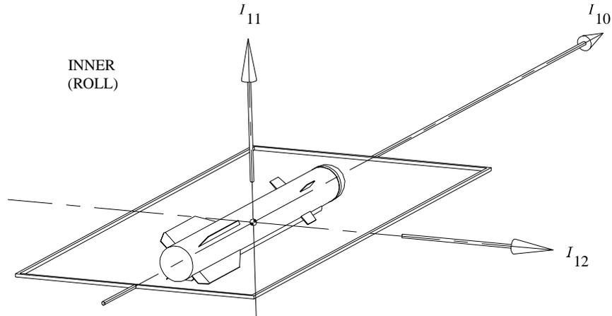
Figure 4-6: Inertia Definition for Inner (Roll) Axis
