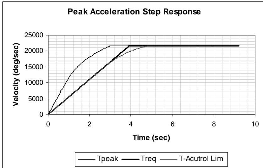
Figure 4-3: Peak Acceleration Step Response for AC130HS High Speed Roll Drive Option
