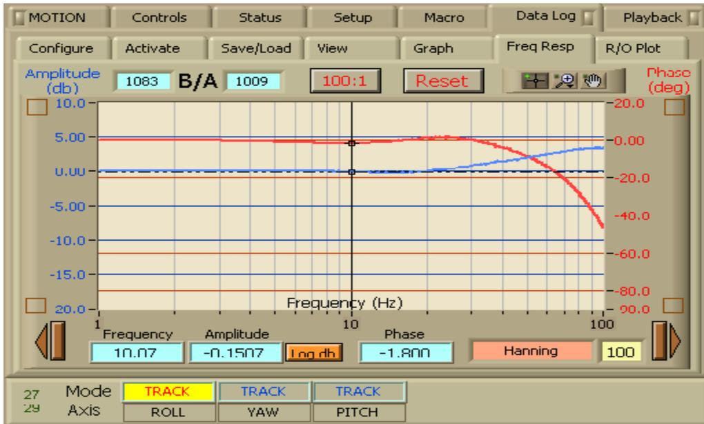
Figure 3. Performance bay roll axis position loop frequency response. Blue trace is gain (scale on left, in dB), red trace is phase (scale on right, in degrees). Cursor is at 10.07 Hz, gain is -0.1507 dB, phase is -1.80 degrees.
