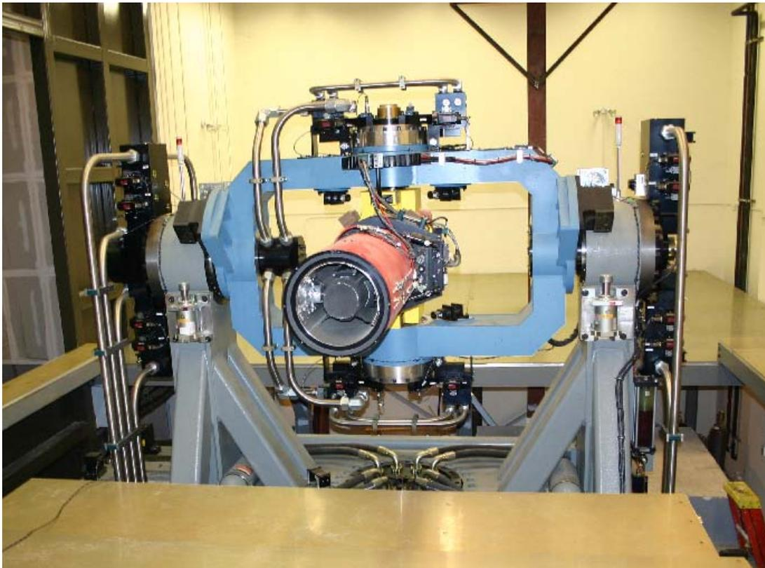
Figure 5. Rear view of production bay FMS, environmental chamber with inert missile installed. FMS base translated from test position and rotated to UUT loading position.
