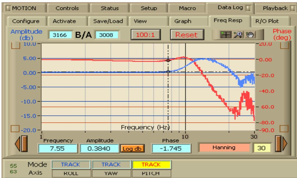
Figure 4. Production bay pitch axis position loop frequency response. Blue trace is gain (scale on left, in dB), red trace is phase (scale on right, in degrees). Cursor is at 7.55 Hz, gain is +0.384 dB, phase is -1.745 degrees.
