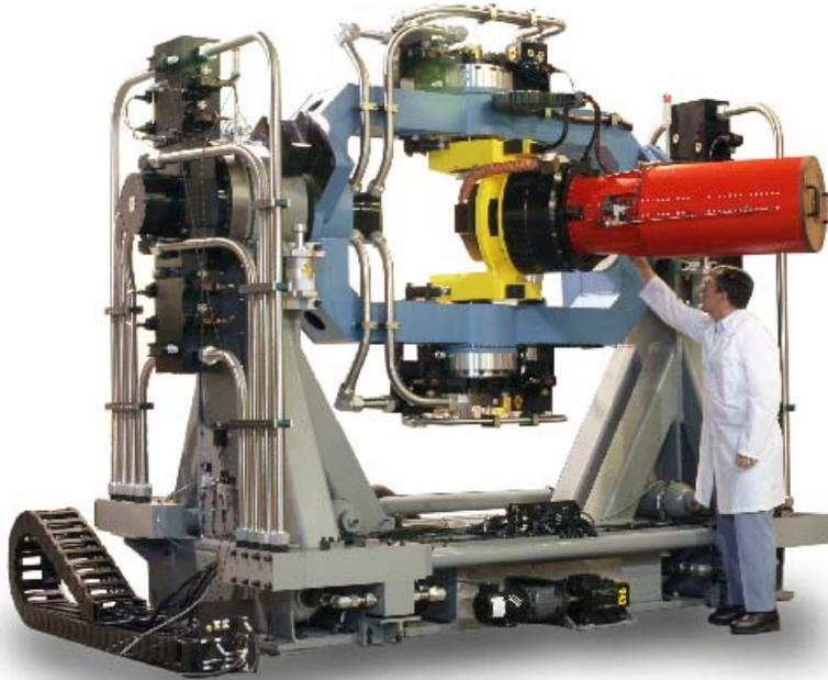
Figure 2. Production bay FMS, showing integrated environmental chamber (red cylinder)
