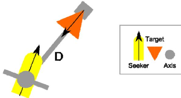
Figure 2: Target and seeker axis, connected with a fixed gimbal system: near field TMS configuration.
