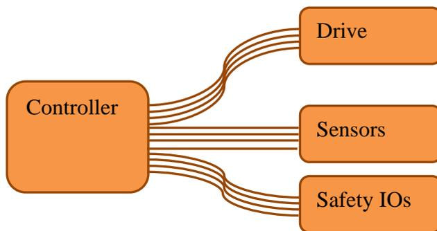
Figure 6: Traditionally connected system with individual connecting wires.
