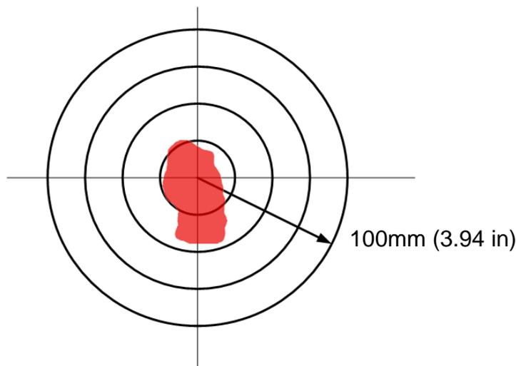
Figure 12: Pointing results are well within the 100mm specification.
