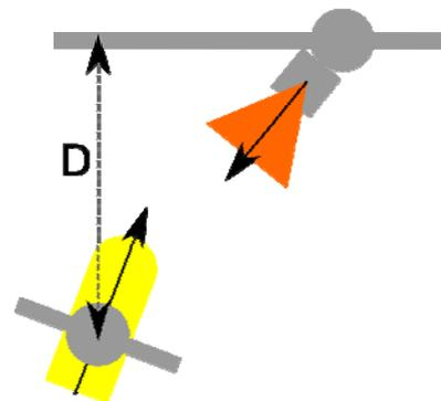
Figure 4: Flat frame TMS. Distance to the target, D, can be varied.
