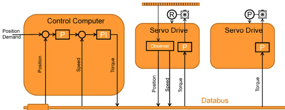
Figure 8: Position, rate and torque loops all closed in the control computer.
