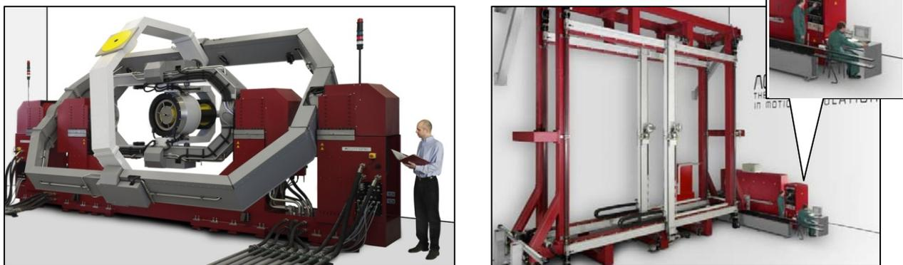
Figure 1: Five axis Hardware-in-the-loop simulator with *near field* TMS is depicted on the left. A DTMS for *far field* target simulation is shown on the right. Observe the persons in the pictures for relative sizes.
