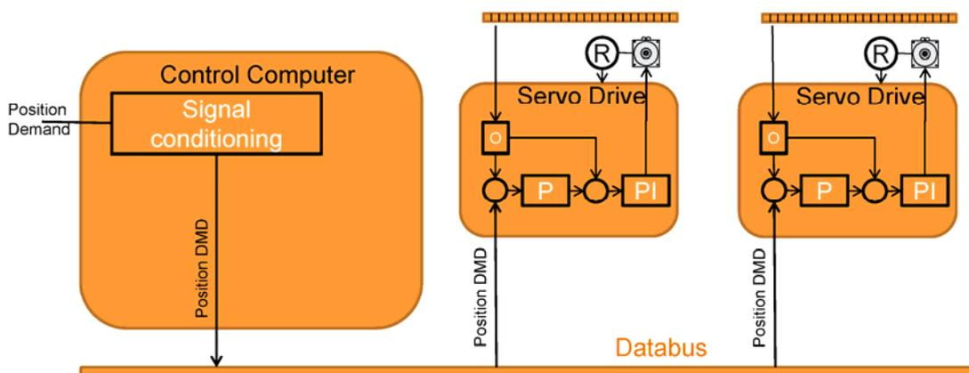
Figure 9: Position, rate and torque loops closed in the individual servo drives.
