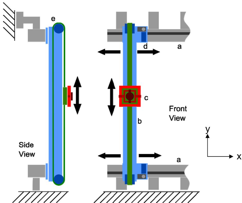
Figure 5: Side view and front view of the TMS. For simplicity a single target.
