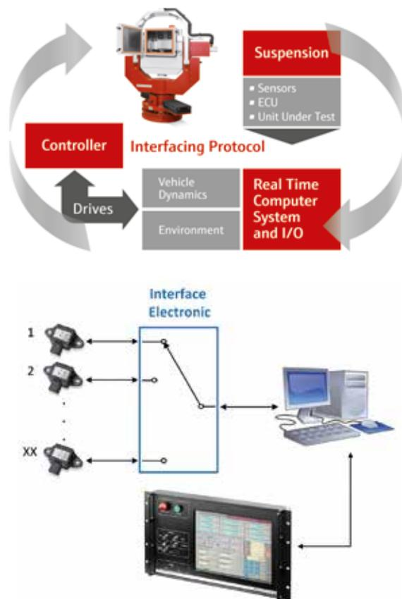
TOP: The basic components of a HIL system
