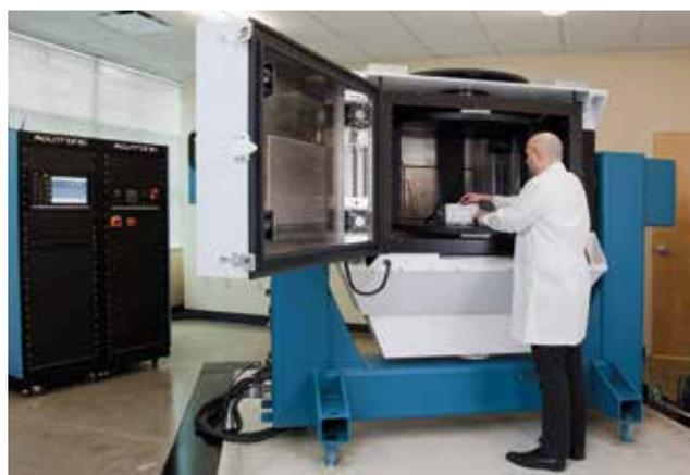
Acutronic's in-house inertial test laboratory can be used by clients for testing and/or calibrating automotive-related motion sensors such as gyros, accelerometers and/or IMUs
